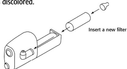
Remove water-trap assembly from the analyzer as shown above. Remove the filter and plastic holder from the housing. Discard the filter element but keep the holder to fit to the new filter. Clean the inside of the filter housing with a suitable soft cloth. Fit the holder onto the new filter element and then insert into the housing. Refit the housing onto the analyzer.
